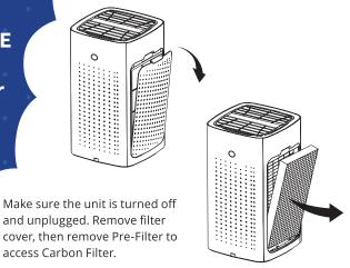
Remove protective bag from Carbon Filter, then reinstall.
